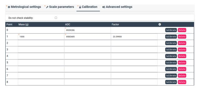
The first step of calibration is always the zero-point calibration.
